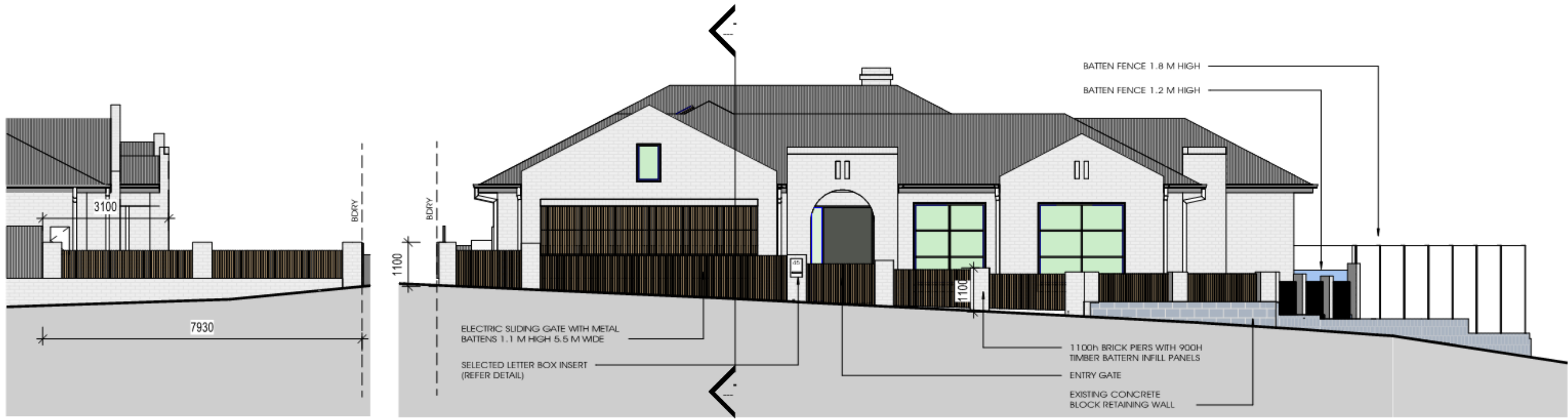
3 Front Fence Elevation - Side 1 : 100
