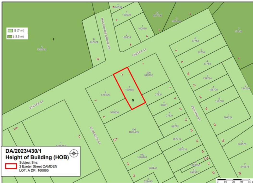
Image 2 – The site is located in an area where the maximum prescribed building height is 7m
