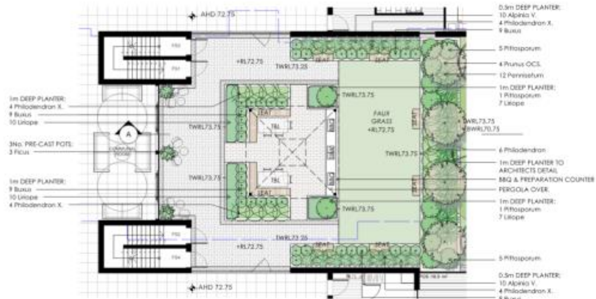
02 Ground Floor Common Open Space 1:100
