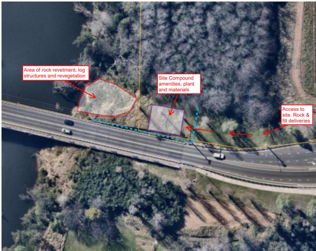
Site 6 – Works involve filling of bank scour area, installation of rock revetment, log structures at river edge and planting. Following concept design is indicative and detailed design will have to be undertaken.
