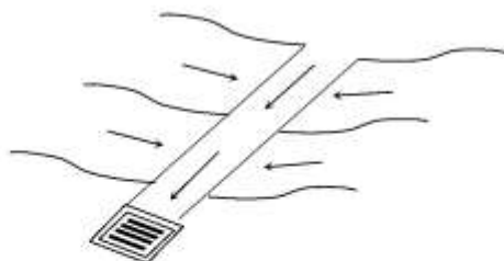
Figure 24.11 A typical mowable swale with water running into a grated sump.
