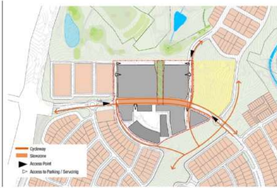
Figure 4: Access configurations and cycleway provision
