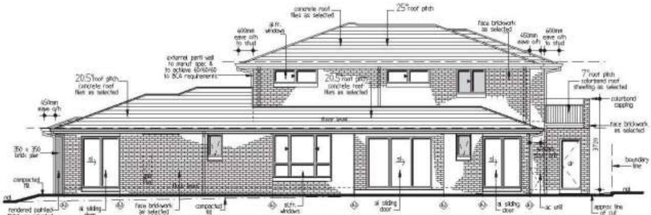
SOUTH WEST ELEVATION 1:100
