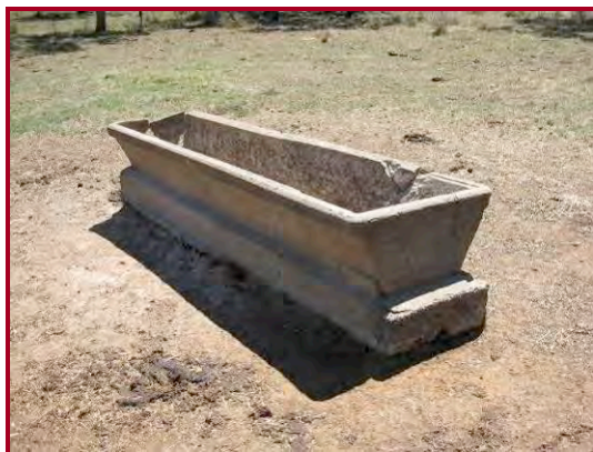
Figure 23. A reinforced concrete trough.
