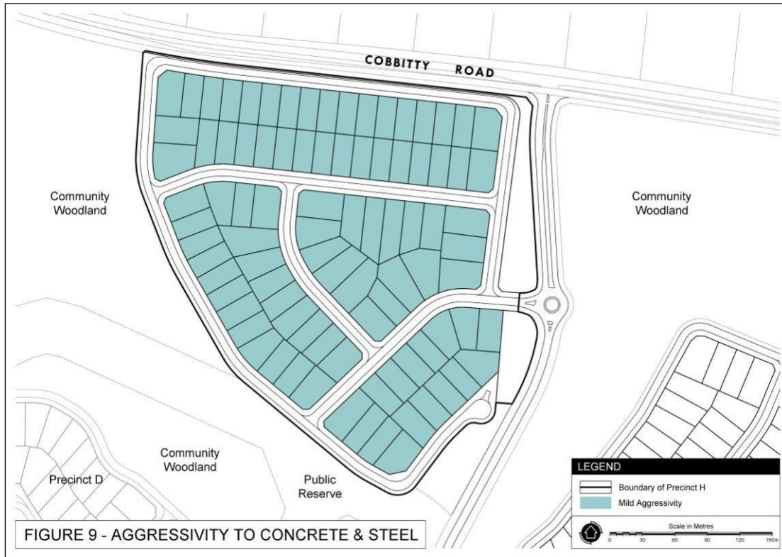
Figure 4-37: Aggressivity to Concrete and Steel in Precinct H Figure 4-37: Aggressivity to Concrete and Steel in Precinct H
