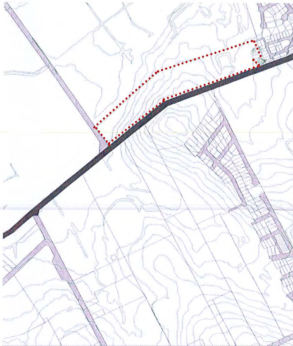
A contour map of the subject site and surrounding land, indicating the nature of the low lying flood plain and gentle rise of the hill on which the main cottage and group of outbuildings have been constructed.
